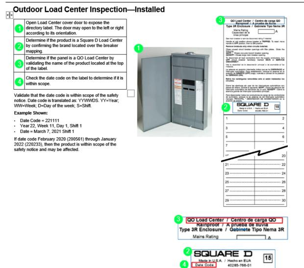
20) How can the date code be found on an affected installed load center (Qualified Personnel)
