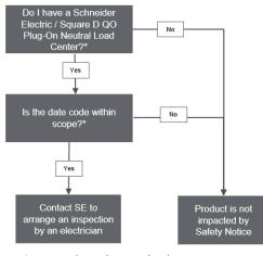
\*Instructions how to determine if you have a Square D QO Plug-On Neutral Load Center and locate the date code can be found on this letter or visit : http://se.com/us/qoloadcenter-safetyrecalInotice
